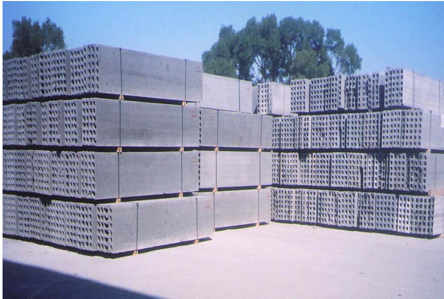
Machine produced Lightweight partition panels
