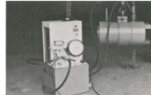
Multistrands stressing jack and hydraulic pump
